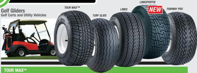
The Tour Max is a low profile, smooth riding tire designed primarily for golf cars and closed community vehicles. The tread pattern, rubber compound, and tire construction provide durability as well as ride comfort on hard surface paths.
